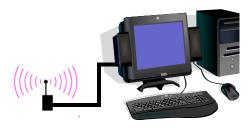
For most effective communications, there must be a clear *visual* line of sight between the transmitter and receiver antennas.
